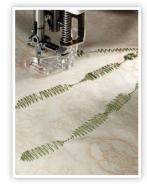
of control of the stitch width. Begin with a straight stitch, then while the machine is still running, press against the knee lifter to widen your stitch to a 9 mm zigzag. Release pressure to gradually return to a straight stitch for a tapered finish. This advanced feature opens up amazing new possibilities for creation expression with free motion quilting, thread painting, raw edge appliqué, free motion monogramming, and more.
