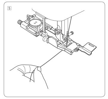
Lower the presser foot and pull the buttonhole lever down as far as it will go.
