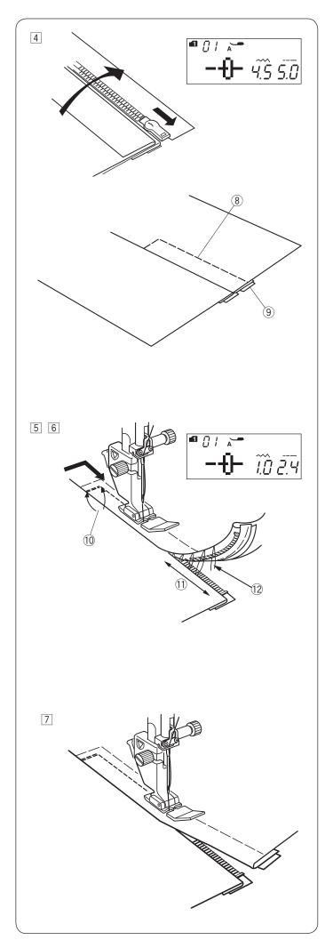
4 Close the zipper and spread the fabric open flat with the right side facing up. Attach the Zigzag foot A.
