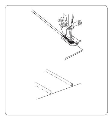
Fold the fabric with the wrong sides together. Place the folded fabric under the blind hem foot. Align the edge of the fold with the guide on the foot, and lower the foot.
