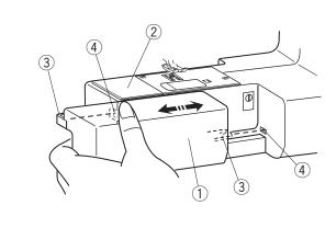
Detaching the table Pull the table away from the machine, as illustrated.
