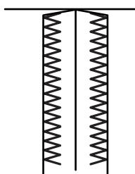
Simple zigzag stitching is used for finishing raw seam edges (overcasting) on most woven fabrics to prevent fabric from unraveling. This is the fastest way to finish an edge.
