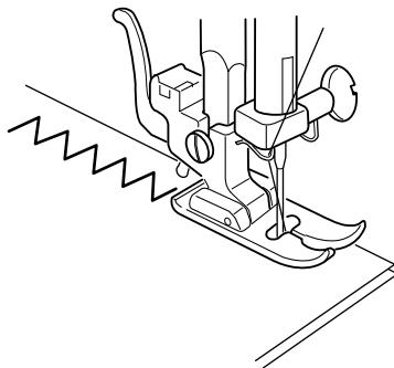
The zigzag stitch is one of the most common and versatile stitches. It can be a utility stitch for button sewing, buttonhole making, hemming, overcasting, mending and darning.
