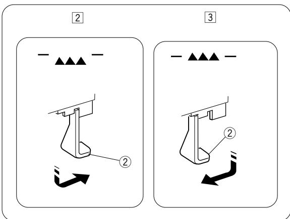
3] To raise the feed dogs, push the lever in the direction of the arrow, as illustrated, and turn handwheel towards you. Feed dogs must be up for normal sewing.
