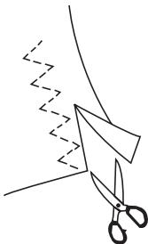
This stitch is used to finish the raw edge on synthetics and other fabrics that tend to pucker. Place your fabric to allow a 1.6 cm (5/8") seam. Trim the seam allowance after sewing. Be careful not to cut the stitches.
