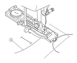
2 Start the machine and sew the buttonhole. Each side of the buttonhole and the bartacks will be sewn over the cord.
