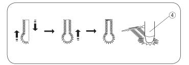
The sewing procedure is the same as the square buttonhole. Use the seam ripper and an eyelet punch ④ to open the buttonhole.
