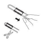
3 Pull the loose ends of the filler cord to tighten it.
