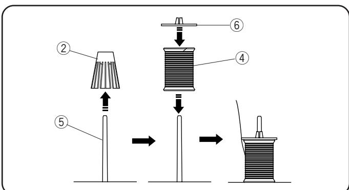
When using small spools, remove the spool holders from the spool pins.
