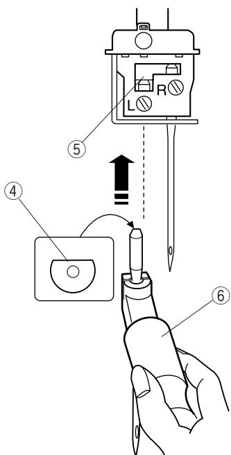
Insert a new needle into the needle clamp with the flat side to the back and push it up against the stopper, then tighten the needle clamp screw.
