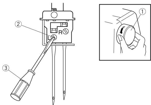
Turn the handwheel toward you to raise the needle to its highest position.
