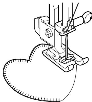
Place the applique on the fabric and baste it in place. Sew, guiding the edge of the applique along the slit on the foot, so that the needle falls off the edge of the applique when it swings to the right.
