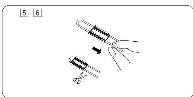
[5] Remove the fabric from the machine and cut the sewing threads.
