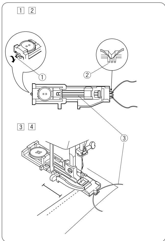
[1] With the automatic buttonhole foot R raised, hook the filler cord on the spur on the back of the buttonhole foot.
