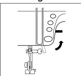
Raise the presser foot. Press the needle up/down button to raise the thread take-up lever to its highest position.
