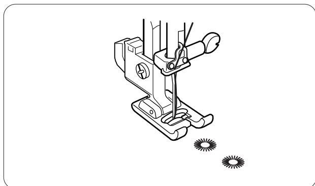
The eyelet is used for belt holes etc.
