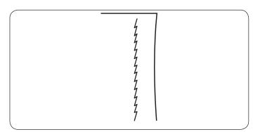
This stitch is a narrow stretch stitch designed to eliminate puckering on knit fabrics and bias seams, while permitting the seam to be pressed completely open flat. Use this stitch for seaming fine fabrics.
