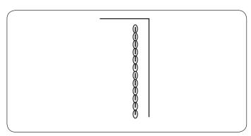
This strong, durable stitch is recommended when both elasticity and strength are necessary in order to insure comfort and durability. Use it to reinforce areas such as crotch and armhole seams. Also use for extra reinforcement when constructing items such as backpacks.
