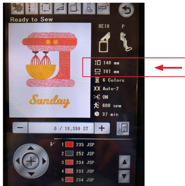
Divide the height (140mm) in half to establish the center. In our sample, the center of the design is 70mm from the upper or lower edge of the design.
