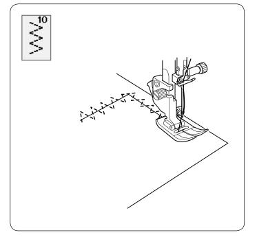
U10 Multiple zigzag stitches These stitches are used for mending tears.
