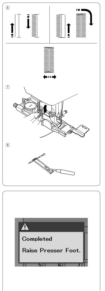
6 The buttonhole is sewn automatically in the sequence shown. When the buttonhole is finished, the machine will stop automatically with the needle in the up position. Press the thread cutter button and remove the fabric.
