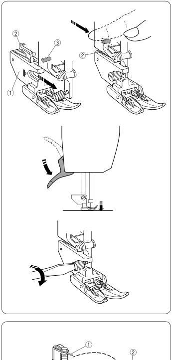
Attaching the Dual Feed Foot Attach the dual feed holder to the presser bar. 1 Dual feed holder
