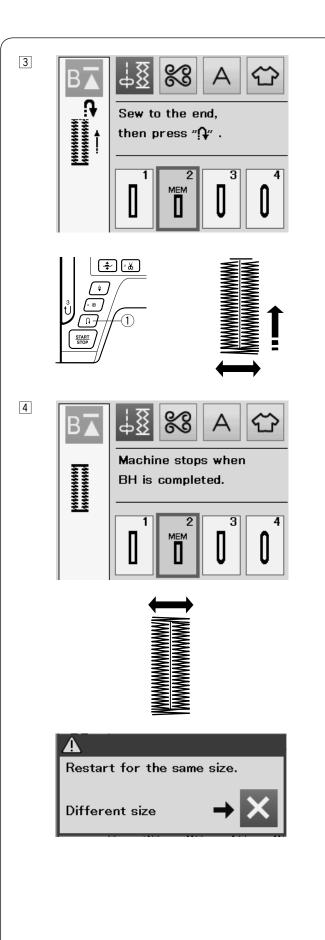
Start sewing again, and the machine sews the front bartack and right side of the buttonhole.
