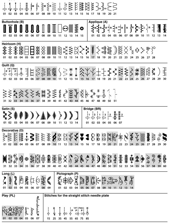
\* Stitch patterns marked with grey can be flipped vertically. (Horizontal mirror image)
