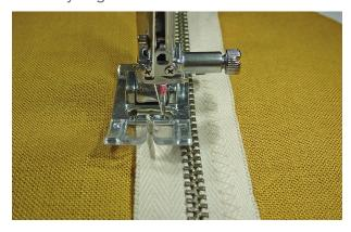
As with most zipper installations, you will need to stop, with the needle in the down position, and open and close the zipper as needed to allow the presser foot to pass the zipper pull.
